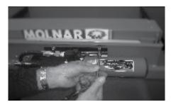
5 Gently holding the pump unit, loosen the bottom left mounting bolt until the pump is free of the main body. Slowly rotate the pump towards you until pump lifts off. Do not disconnect the pump delivery hose.
