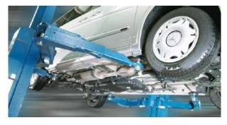
The long reach allows the operator to extend out the arms to pick up points on very long vehicles where stability can be maximised and as such, the lifting safety is vastly increased.
