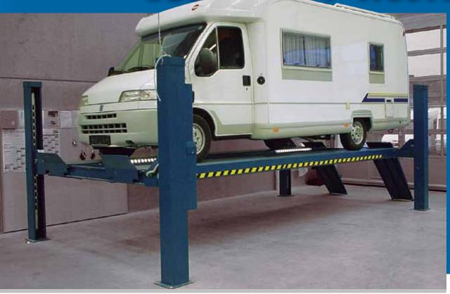
Combi Lift is versatility and stability. Fully optioned, the Combi Lift is the lift able to handle almost any vehicle service or repair requirement. The 4 post hoist configuration provides more support under a vehicle when servicing making it an inherently safer design especially for larger vehicles or vehicles with uneven weight distributions. The 6500kg capacity and the width adjustable runways will allow for a great range of vehicles in size and weight.
