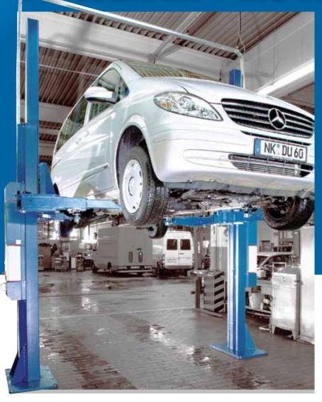
The 2.60 SST DG is not only one of the most innovative hoists utilising Nussbaum's SST proprietary technology but it is also one of the most adaptable 2 post hoists. With Nussbaum's doublejointed arms system, the arms fold inwards to easily reach the pickup points on
