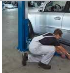
Telescopic lifting arms and very low lifting point
