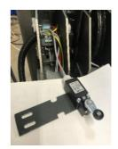
3. Use the same holes from the removed S13-switch to install the metal bracket (474626) with switch.
