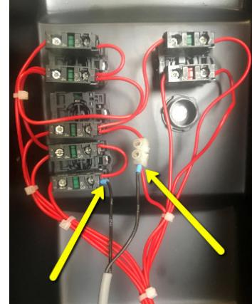
button and connect it to the cable connector:
