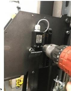
2. Drill a 4,2 mm hole in the bottom right S23 switch hole and make a M5 thread. Install a screw (253595) in the new tread.
