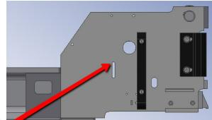
Use the existing machined slot to install a screw (253595) washer (214771) and nut (240306) in the left switch hole.
