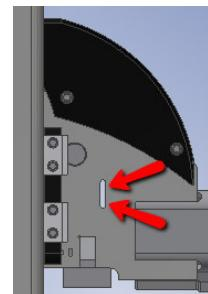
3. Use the existing machined slot outside on the main cross beams front right side: Install the max deviation bracket (609366) with bracket (474627) and two screw (254646).
